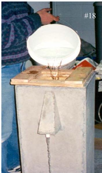
Note: The tall wood box type diffuser or the plastic bucket diffuser used with the double lid are the BEST type of diffuser lid assemblies.
