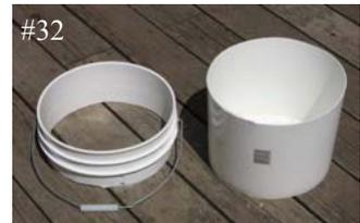
31. A line 3 cm below mark is drawn around bucket to guide cutting the bucket down with a saw or sharp knife. This will allow for the spacer sticks (see below) and the thickness of the lid.
