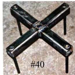
40 – 42. Details of interior mold puller.
