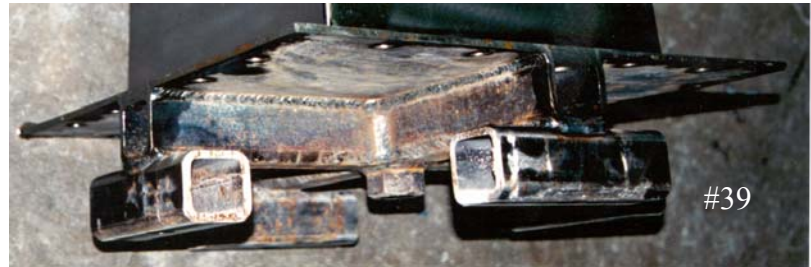
39. Side view of foot on bottom of interior mold.
