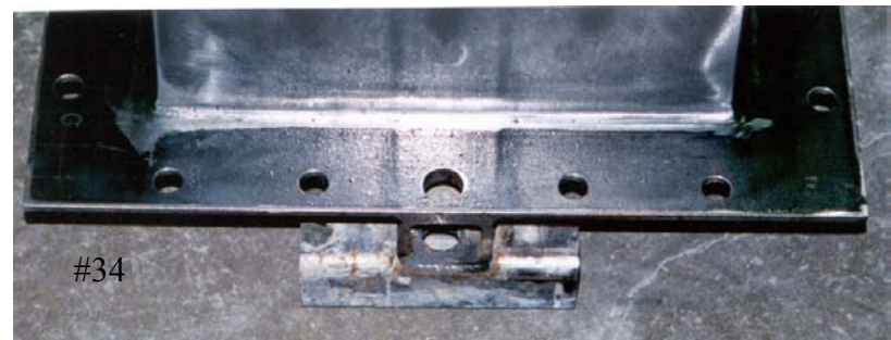
347. Details of foot at bottom of interior mold.
