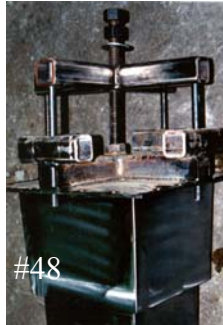
48 – 54. Note use of puller and the puller bolt to remove the interior mold.
